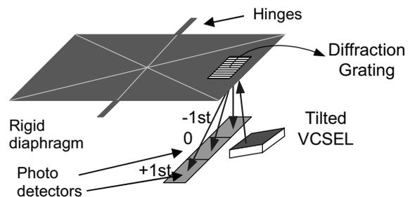
Figure 1. Schematic of a micromachined directional microphone with integrated optical readout.
