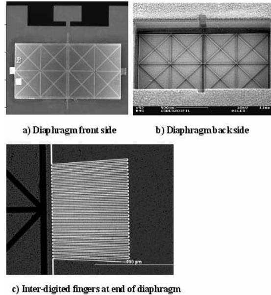
Figure 3. Fabricated differential microphone diaphragm with inter-digitated fingers a) Front side optical view. b) Backside view using an SEM. c) Inter-digitated fingers at the end of the diaphragm with backside illumination.
