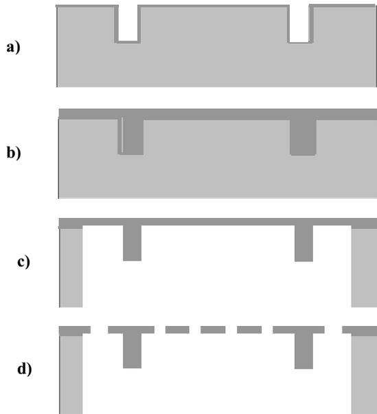
Figure 2. Fabrication process flow for the differential microphone diaphragm with inter-digitated fingers at the ends. a) Deep RIE and thermal oxide growth. b) Polysilicon deposition and chemical mechanical polish. c) Backside RIE and thermal oxide removal. d) Polysilicon RIE for fingers and slits.
