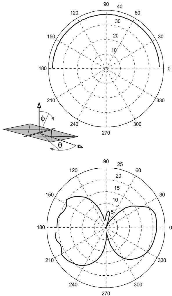
Figure 5. Variation of acoustic response (in dB) of the microphone measured at 2 kHz. Top: Device response in the  $\phi$  direction showing expected omnidirectional behavior. Bottom: Variation of device response in the  $\theta$  direction showing expected figure-8 behavior.
